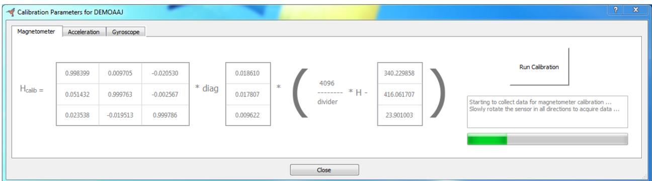
If you want to calibrate the magnetometers, press the “Run Calibration” button. Then you have to turn the sensor in smooth motions, so that as many different angles as possible can be measured. If the calibration was successful, the parameters can be stored to the sensor or dropped otherwise.
