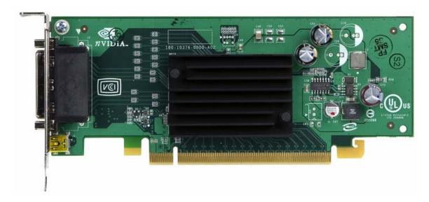
Figure 2. NVIDIA Quadro Plex Interface Card with Low Profile Bracket
