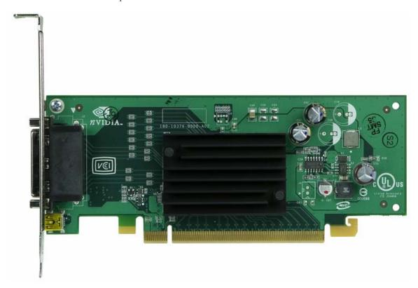
Figure 1. NVIDIA Quadro Plex Interface Card with Standard Bracket
