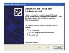
3 Insert the installation CD for the drivers included in the Tesla C2050 package. Follow instructions in the installer package.
