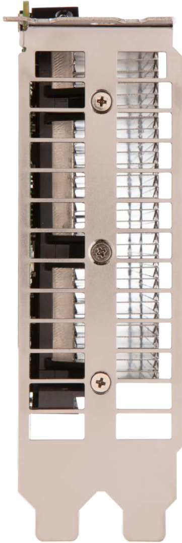
Figure 3. Tesla K20 Bracket
