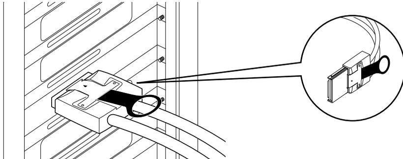
3. Connect the other end of the cable to the back of the Tesla system. The thumb tabs on the cable should face outward for the cable to engage properly.
