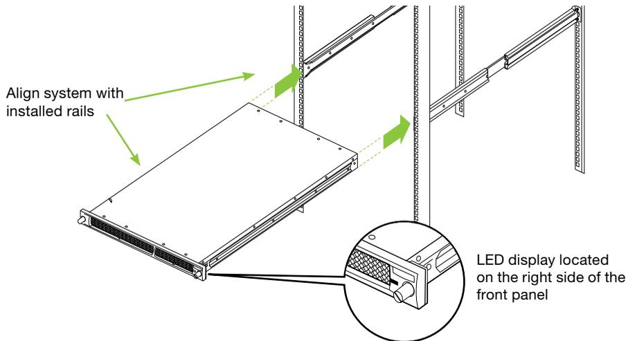
10. Make sure the status LED on the front panel of the system is located on the right side for proper installation.
