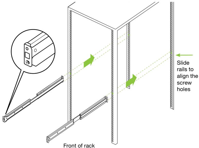
5. Slide the rail onto rack post. The studs in the front and back should hold the rail in place temporarily.
