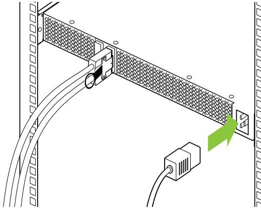
5. Plug the power cord from the Tesla system to an AC outlet (it is recommended to use a power surge protected outlet).
