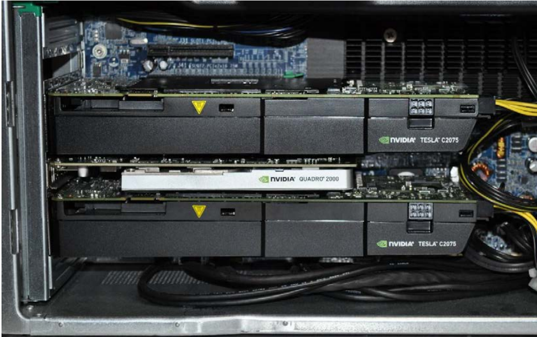
Figure 6. Workstation Configured with One Quadro and Two Tesla Cards
