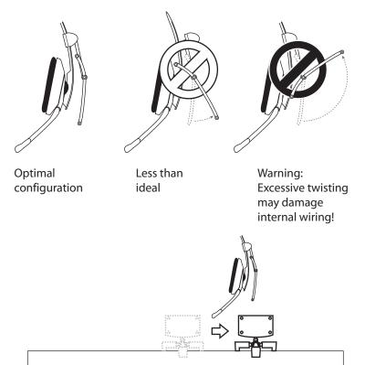
Optimally, position the TrackIR on left side of your monitor until it is centered with TrackClip PRO's LEDs.
