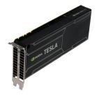
Based on DGEMM performance: Tesla M2090 = 410 gigaflops, Tesla K40 > 1000 gigaflops
