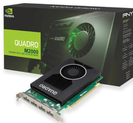
This advanced graphics card features an NVIDIA Maxwell™- based GPU, plus 4 GB of ultra-fast on-board memory and the power to drive four 4K displays natively. This makes it an excellent choice for accelerating product development and content creation workflows that demand fluid interactivity with complex models and scenes. Creative professionals can tap into this increased performance—as well as hardware HEVC encode and decode engines—to accelerate both creation and playback of HEVC content.
